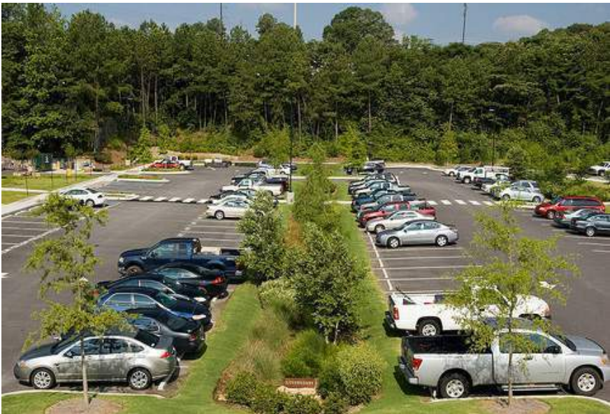
A central landscaped swale absorbs rainwater and adds visual interest
