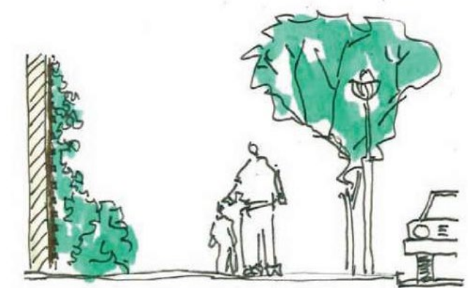
When blank walls are unavoidable, they should be screened with planting or treated with special materials
